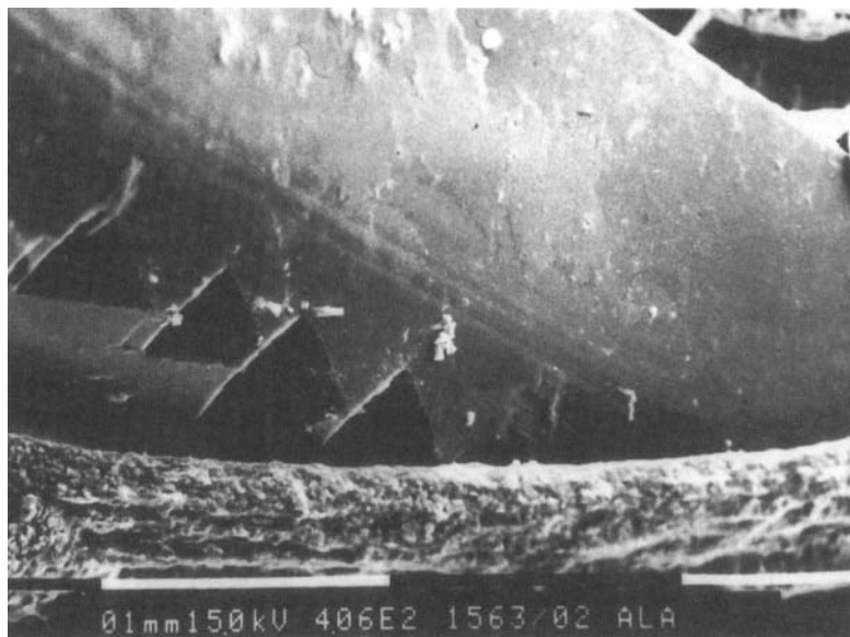
Figure 3.4. Scanning electron micrograph of the \{hk0\} side faces of (D,L)-alanine etched by (L)-threonine; only two faces are shown, one etched and the other smooth.
